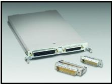
The Model 7709 plug-in module is a two-pole, 6×8 matrix module. It can connect any combination of six differential channels of instrumentation to any combination of eight differential device-under-test channels. The instrumentation can be AC and DC sources, internal or external meters, oscilloscopes, etc. This matrix configuration allows wide flexibility for complex test sys-
